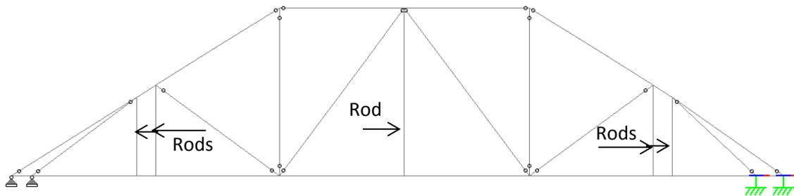
Fig. 5 STAAD two dimensional finite element model of the Moxley Bridge
