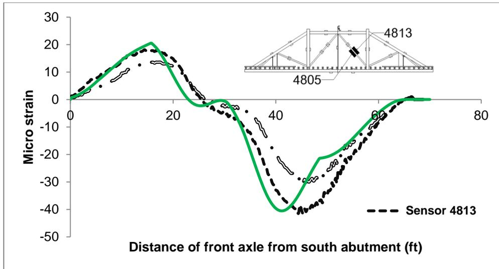
Fig. 7 Analytical and field strains in the diagonal member just to the right of the middle rod
