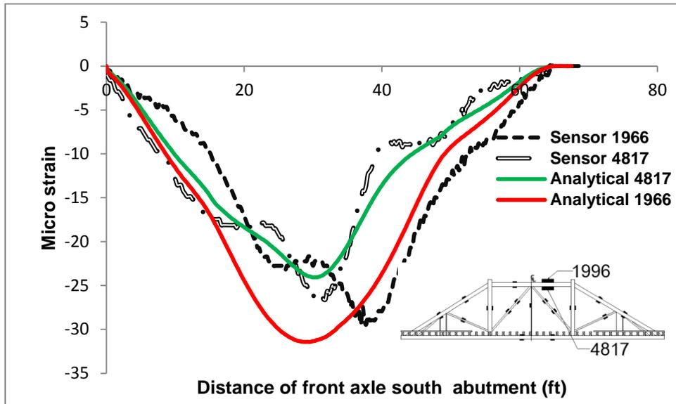
Fig.9 Analytical and field strains the left diagonal member
