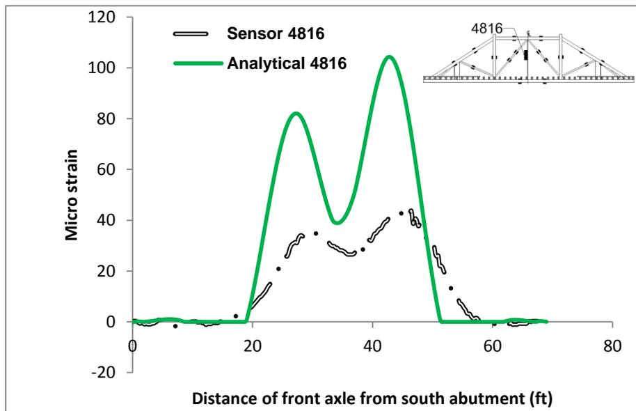
Fig. 10 Analytical and field strains in the middle rod
