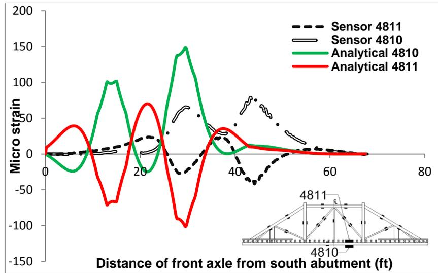
Figure 11 Analytical and field strains in the bottom chord member to the right of the middle rod
