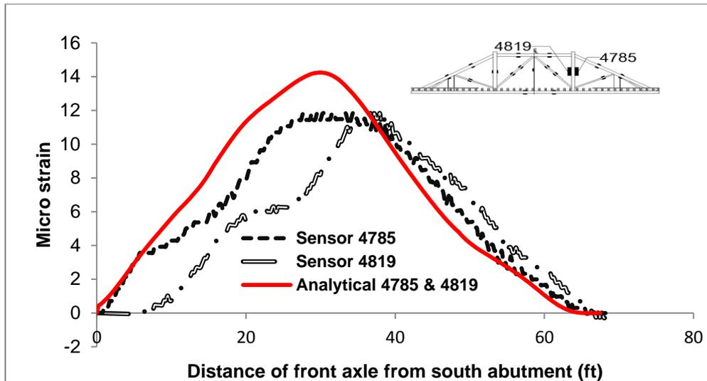
Fig.8 Analytical and field strains in the left timber post
