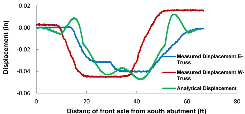
Fig. 6 Variation in the mid-span displacement as the truck travels along the Moxley Bridge
