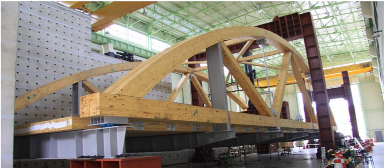
Fig. 3 Static load testing in laboratory
