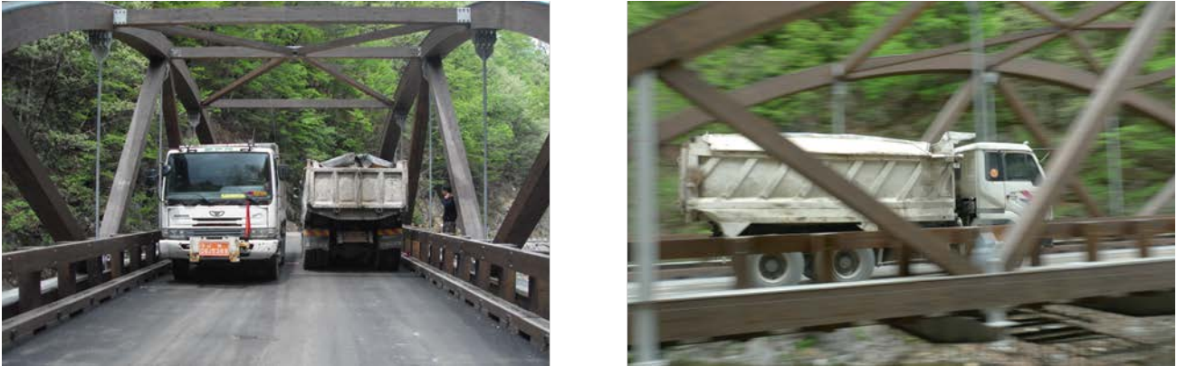
Fig. 9 Truck loading (left : static test, right : dynamic test)
