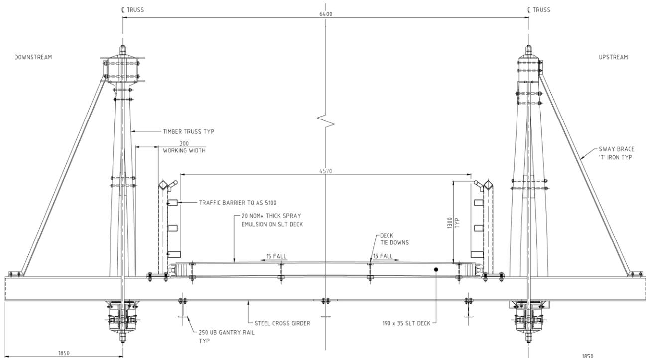
Figure 7 – Typical Cross Section of the new trusses, showing traffic barrier & SLT deck
