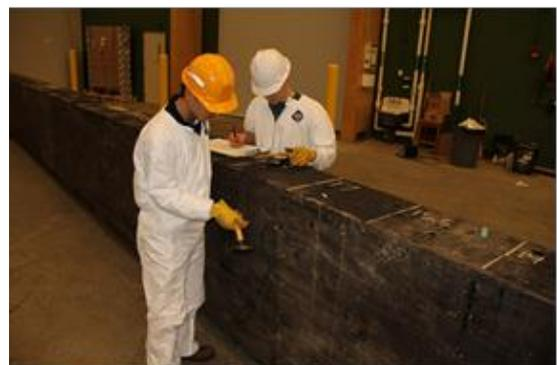
Figure 4. NDE testing is performed in the laboratory to detect internal decay.
