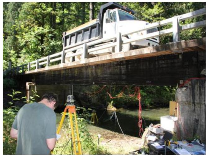
Figure 2. Optical level was also used to collect deflections from calibrated rules suspended from each girder.
