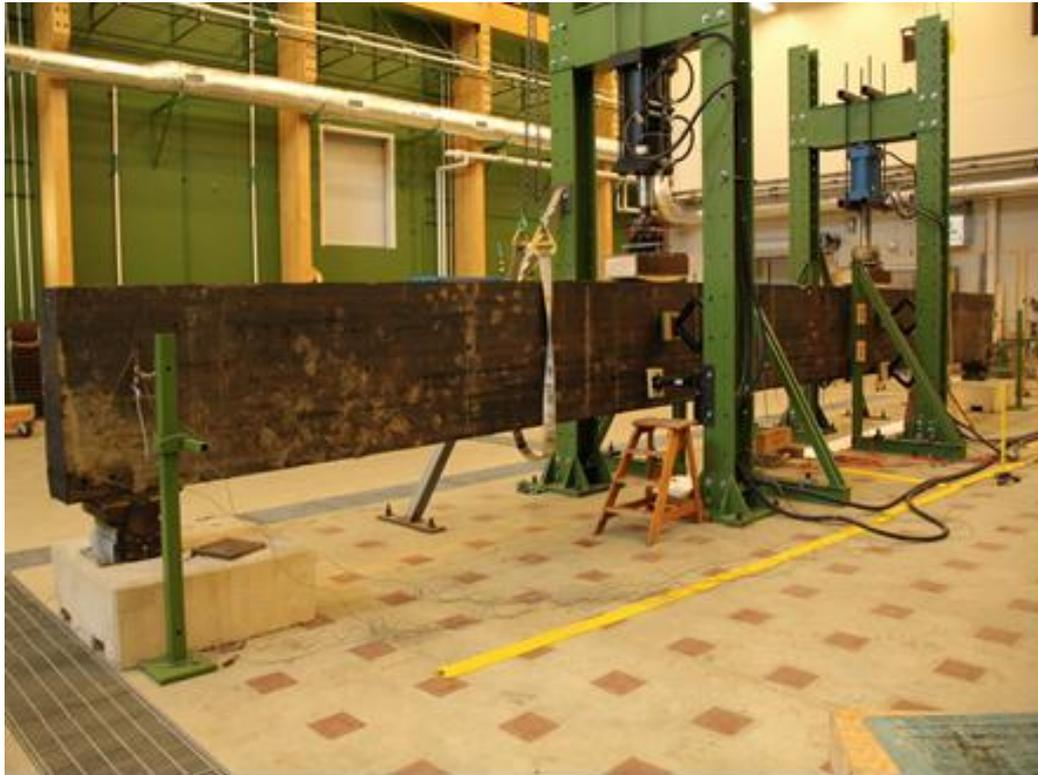
*Figure 5. Static load testing was performed to determine member stiffness and ultimate load capacity of these 60-year-old salvaged glulam girders at the FPL Centennial Research Facility.*
