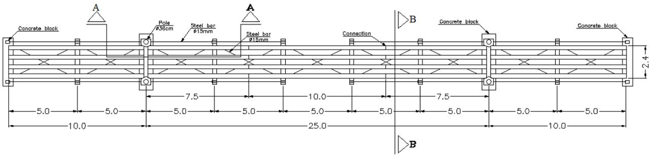
Fig. 2 Bottom view of the footbridge.
