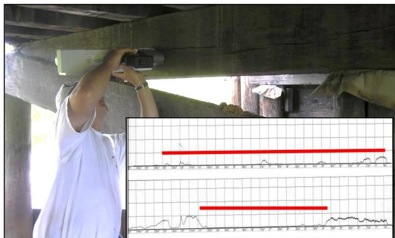
*Figure 5 – Resistance microdrilling techniques were used to inspect timber bridge elements.*
