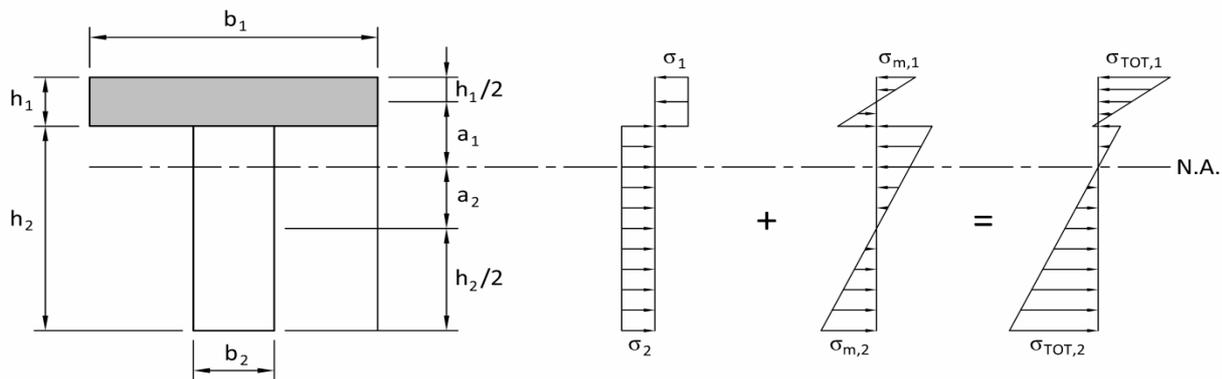
Figure 5 Cross-sectional geometry and stresses according to the  $\gamma$ -method
