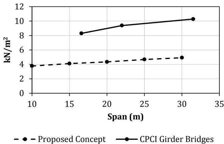
Figure 7 Superstructure weight per unit deck area
