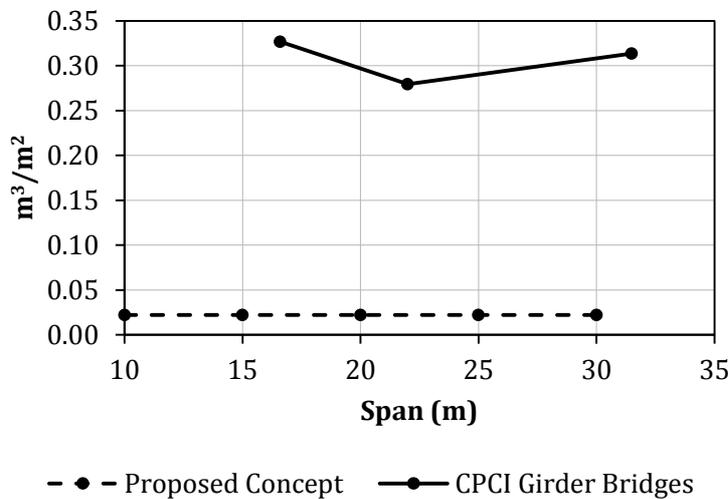
Figure 8 Volume of cast-in-place concrete per unit deck area
