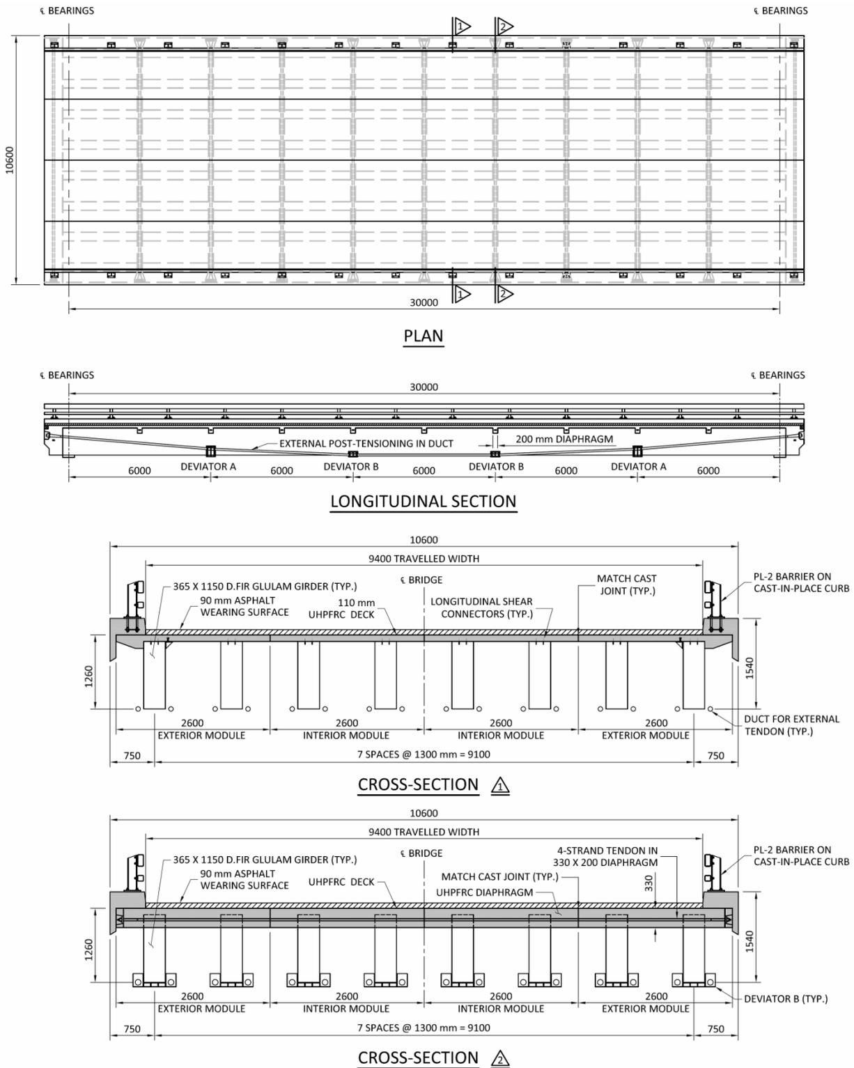
Figure 2 Plan, longitudinal section, and cross-sections for a 30 m span
