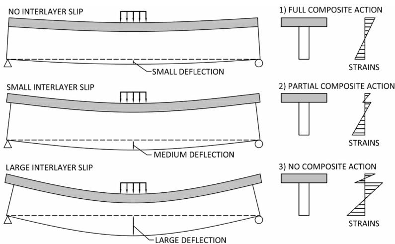
Figure 1 Varying degrees of composite action in a wood-concrete composite system (adapted from [2])
