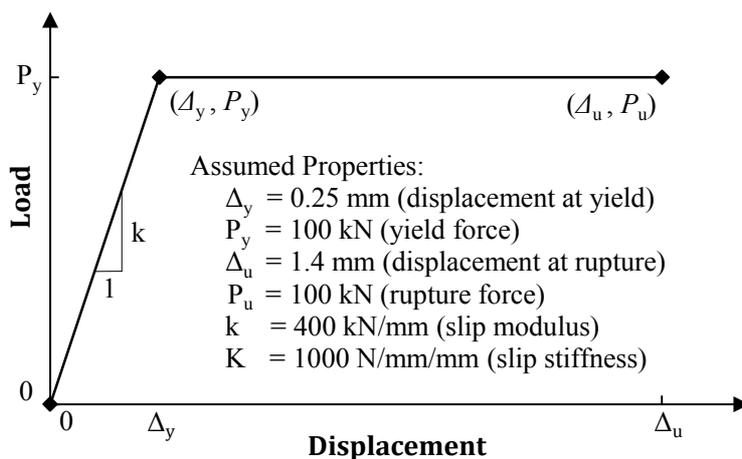
Figure 4 Idealized load-displacement curve for assumed longitudinal shear connector
