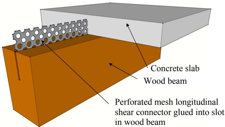
Figure 3 Perforated mild steel mesh longitudinal shear connector (adapted from [13])
