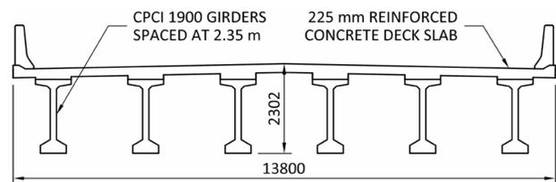
Figure 6 Cross-section of a typical slab-on-CPCI-girder bridge
