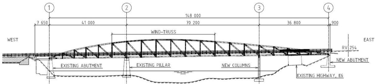
Figure 4 The final shape of the truss
