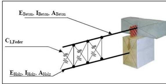
Figure 3: Truss model
