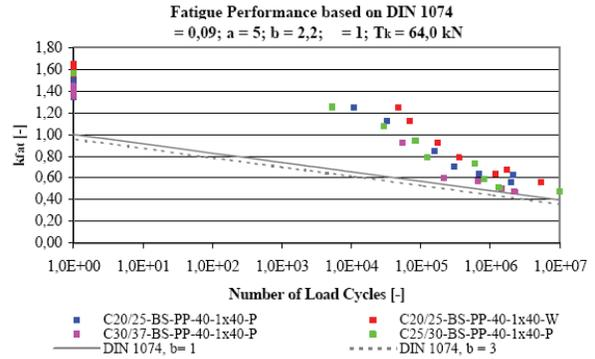
Figure 5: Fatigue analysis vs. test data
